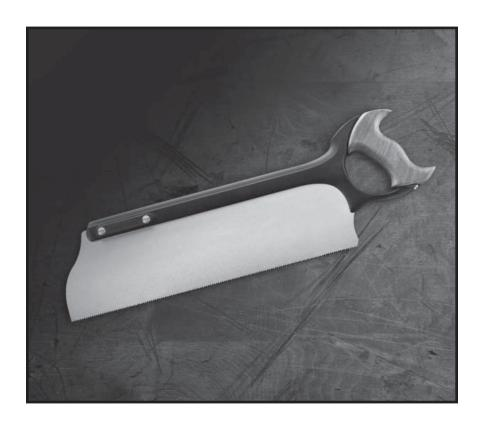
The Veritas® tenon saws combine the best characteristics of the classic fine joinery saw with those of state-of-the-art materials and construction methods. The tooth pattern on the thin high-carbon steel blade provides a good balance between cutting action and surface finish. The design of the wooden handle has been developed to give good power transfer while still allowing a three- or four-finger grip for precise control.
